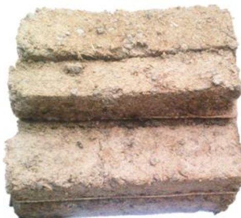
Figure 2: A stark of briquettes produced from sawdust, palm kernel shell and cement.
