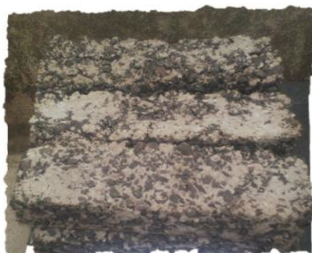
Figure 3: A stark of briquettes produced with palm kernel shell (PKS) and soaked mashed paper.
